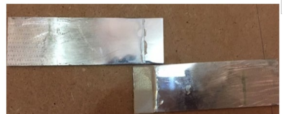
Figure 1: (a) dimensions of test Specimen; and (b) prepared Al specimens according to ASTM D1002
