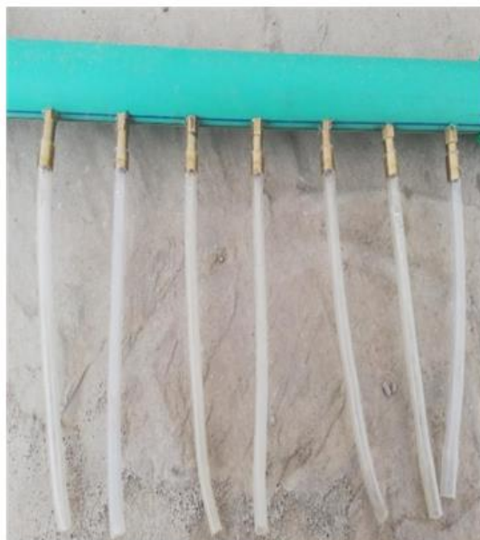
Fig. 2. Tubes used to connect water with PV panel
